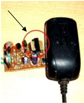
Fig: 16.21 Transformer battery charger
