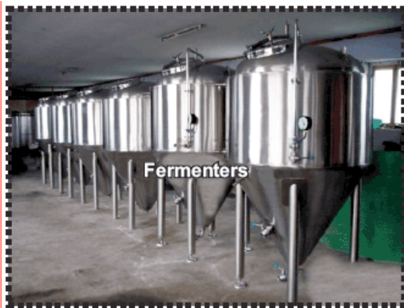
Figure 17.5: Fermenters used in food and pharmaceutical industry
