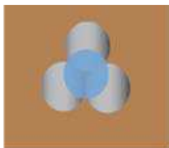
Fig (4.22 c) The formation of a tetrahedral site, due to four balls
