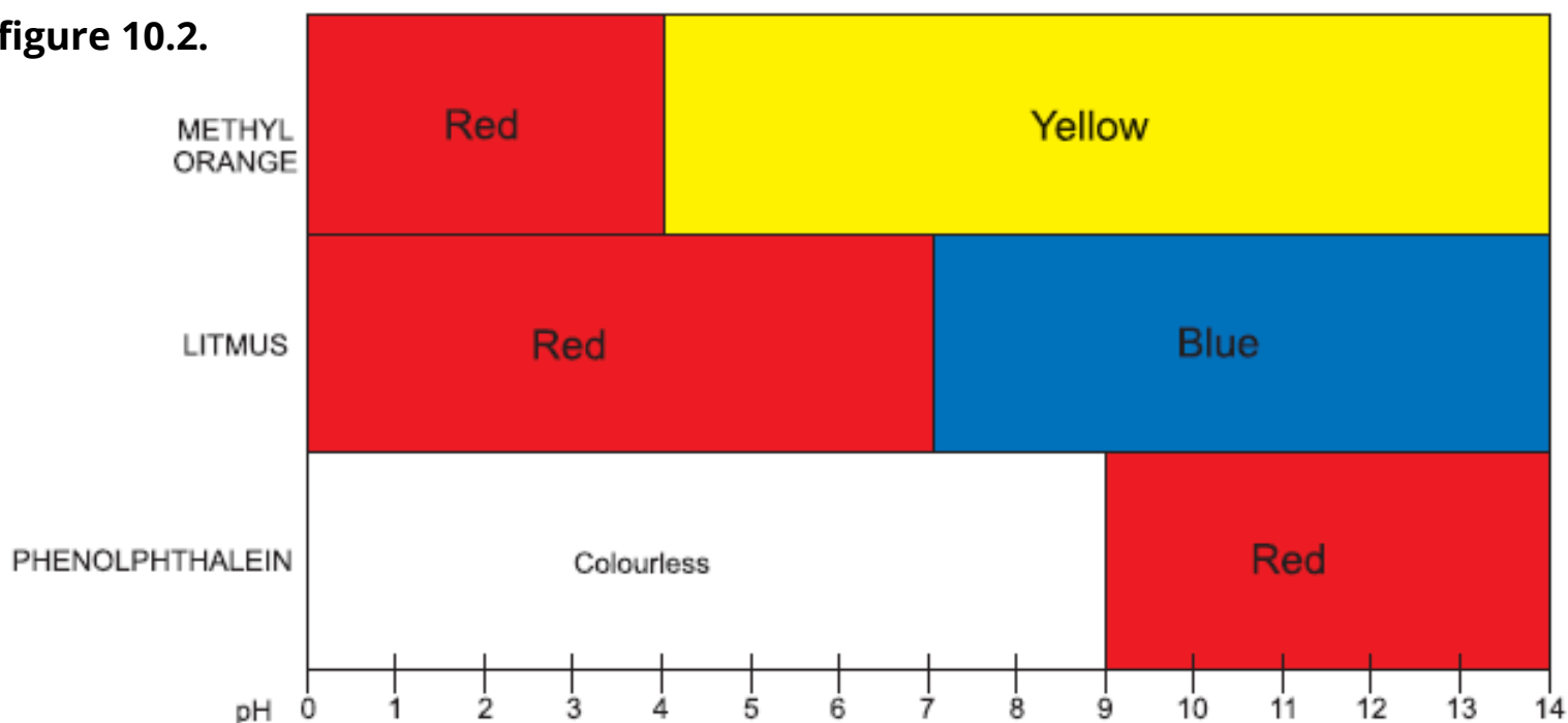
Fig. 10.2. Colours of indicators at different pH solutions
