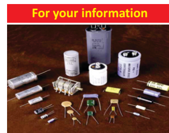
All of these devices are capacitors, which store electric charge and energy.
