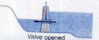
High tide: Water is allowed to flow back into the basin, driving turbines.
