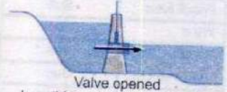
Low tide: Water is beginning to flow out of basin to ocean, driving turbines.
