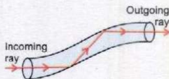
Fig.10.10 (b) Light propagation within a flexible glass fibre.
