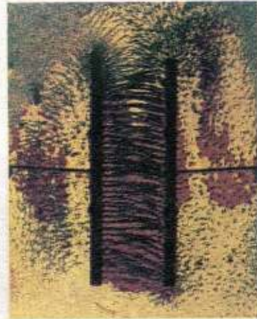
The electric field lines between the plates of a parallel-plate capacitor. Small bits of thread are suspended in oil and become aligned with the electric field. Note that the lines are equally spaced, indicating that the electric field there is uniform.
