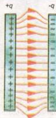
Fig. 12.10 In the central region of a parallel plate capacitor the electric field lines are parallel and evenly spaced, indicating that the electric field there has the same magnitude and direction at all points.
