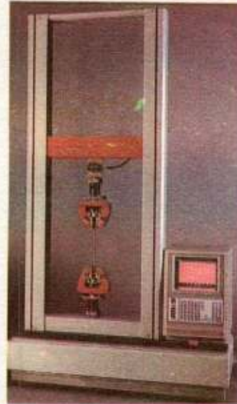
This is a machine used to investigate the way the extension of a material varies with the force stretching it.
