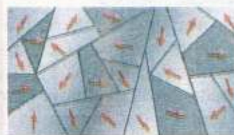
Fig 17.16 Magnetic domains within an unmagnetized ferromagnet.
