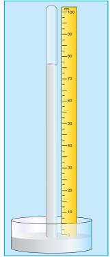
Figure 7.12: A mercury barometer
