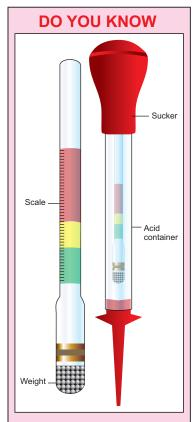
Hydrometer is a glass tube with a scale marked on its stem and heavy weight in the bottom. It is partially immersed in a fluid, the density of which is to be measured. One type of hydrometer is used to measure the concentration of acid in a battery. It is called acid meter.
