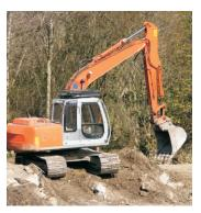
Figure 7.15 Hydraulic excavator
