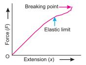
Figure 7.24: Graph between force and extension.
