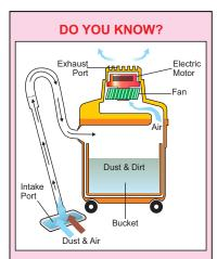
The fan in a vacuum cleaner lowers air pressure in its bucket. The atmospheric air rushes into it carrying dust and dirt with it through its intake port. The dust and dirt particles are blocked by the filter while air escapes out.
