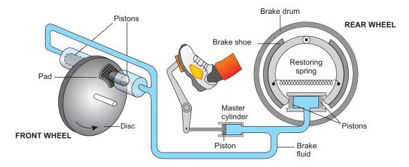
Figure 7.17: A hydraulic brake of a car
